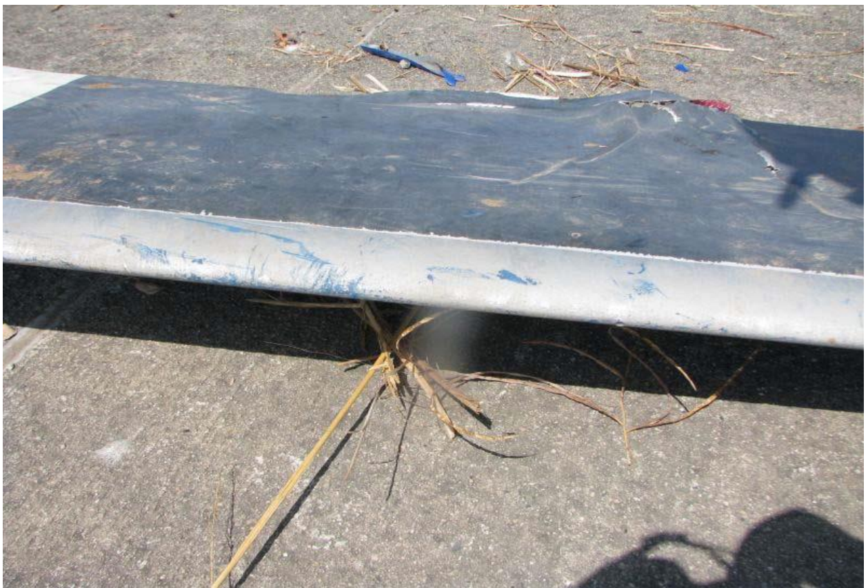
Picture 17 Blue paint transfers consistent with tailboom color on main rotor blade leading edge
