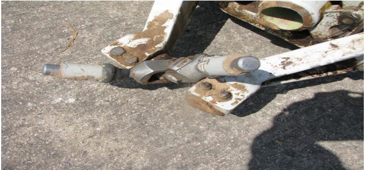
Picture 12. Top end of both pitch change links fractured at clevis inserts consistent with overload
