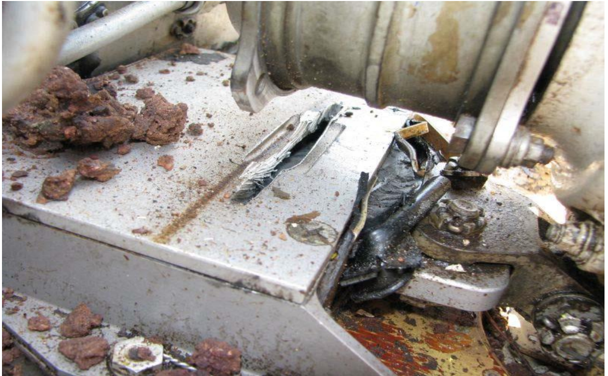
Picture 4 Isolation mount with abraded away material from rotating contact with outer coupling
