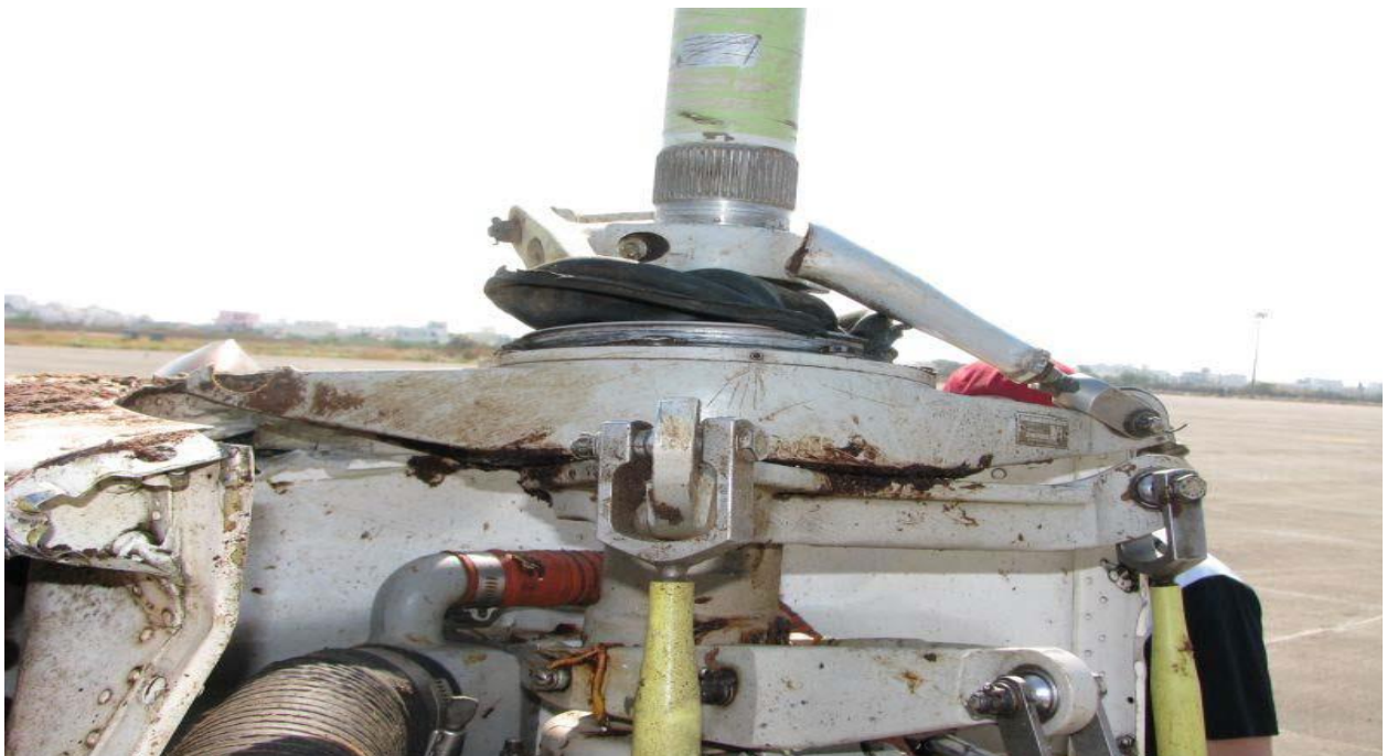
Picture13 Pitch change link (red) and swash plate attachment ear (blue) overload fractures
