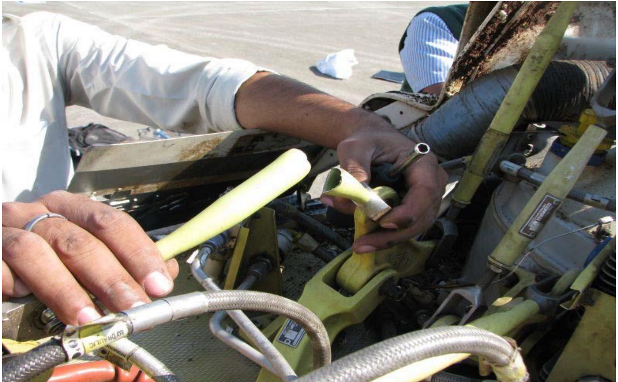
Picture11. Right servo extension tube fractured consistent with bending overload at impact.
