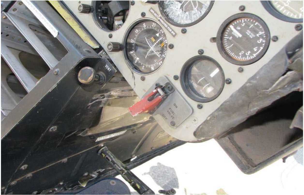
Picture 9 Fuel valve switch in Off position
