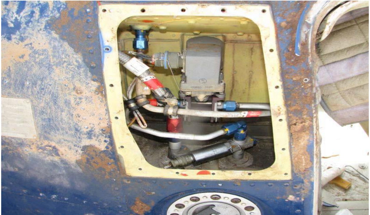
Picture 7 Fuel lines to shut-off valve and fuel pressure transducer were intact
