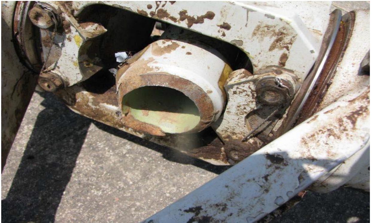
Picture 1 Mast fractured below static stops
