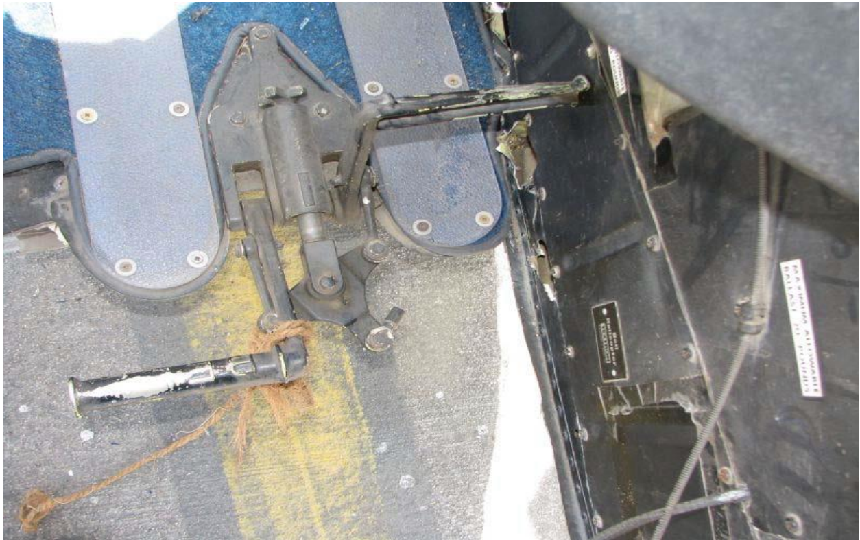
Picture15 Pilot anti-torque pedals intact
