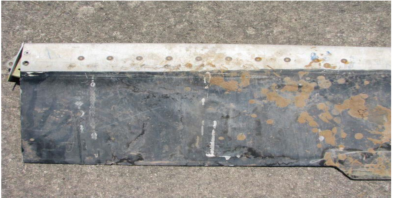
Picture16 Main rotor blade tip section with chordwise markings on bottom of blade
