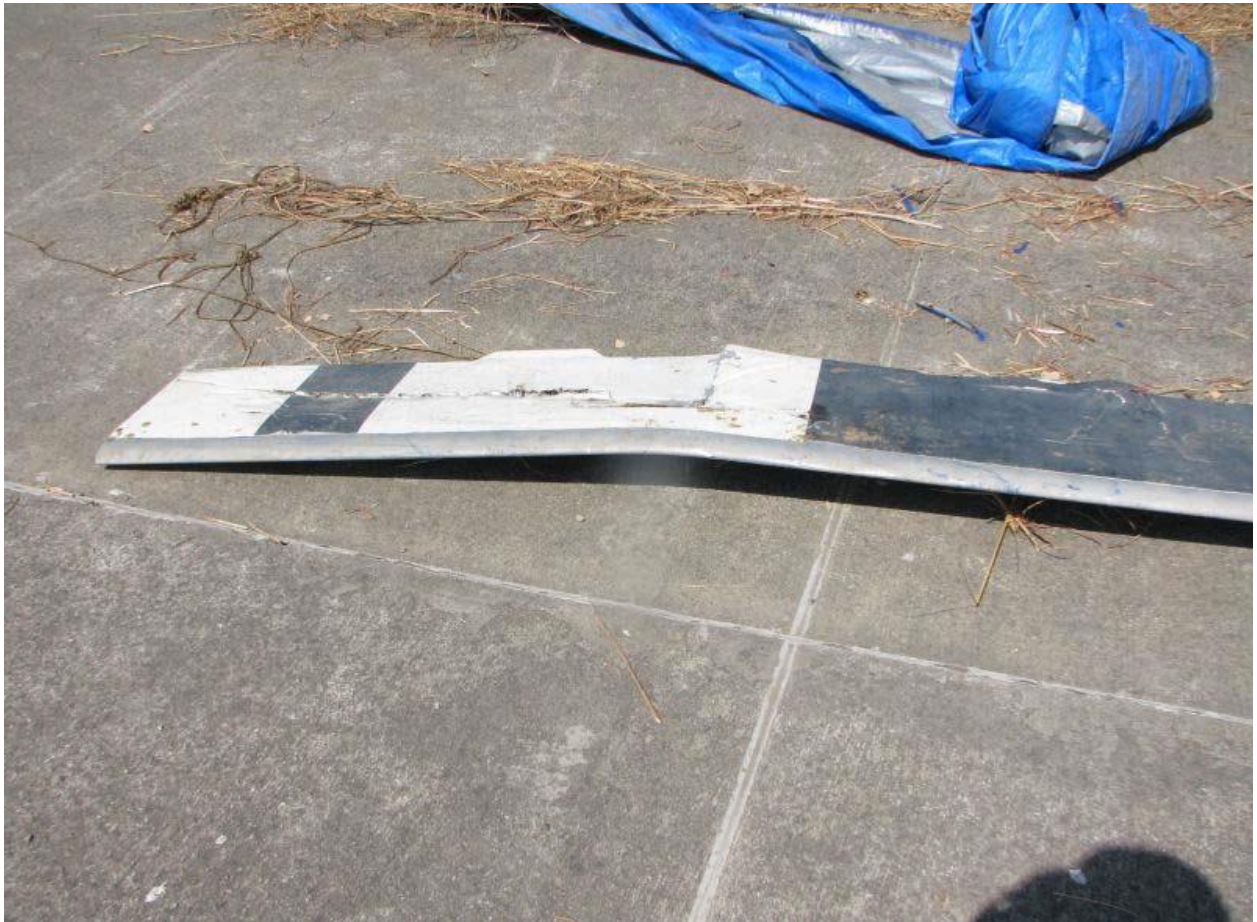
Picture 18 Main rotor blade bent down approx. 3 feet from tip consistent with ground contact
