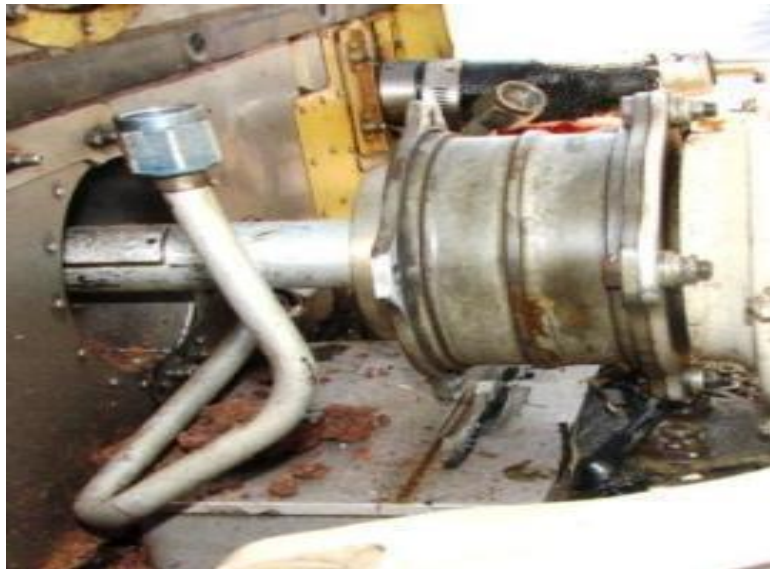
Fuel-Filter 'Pop-Up' Bypass Indicator
