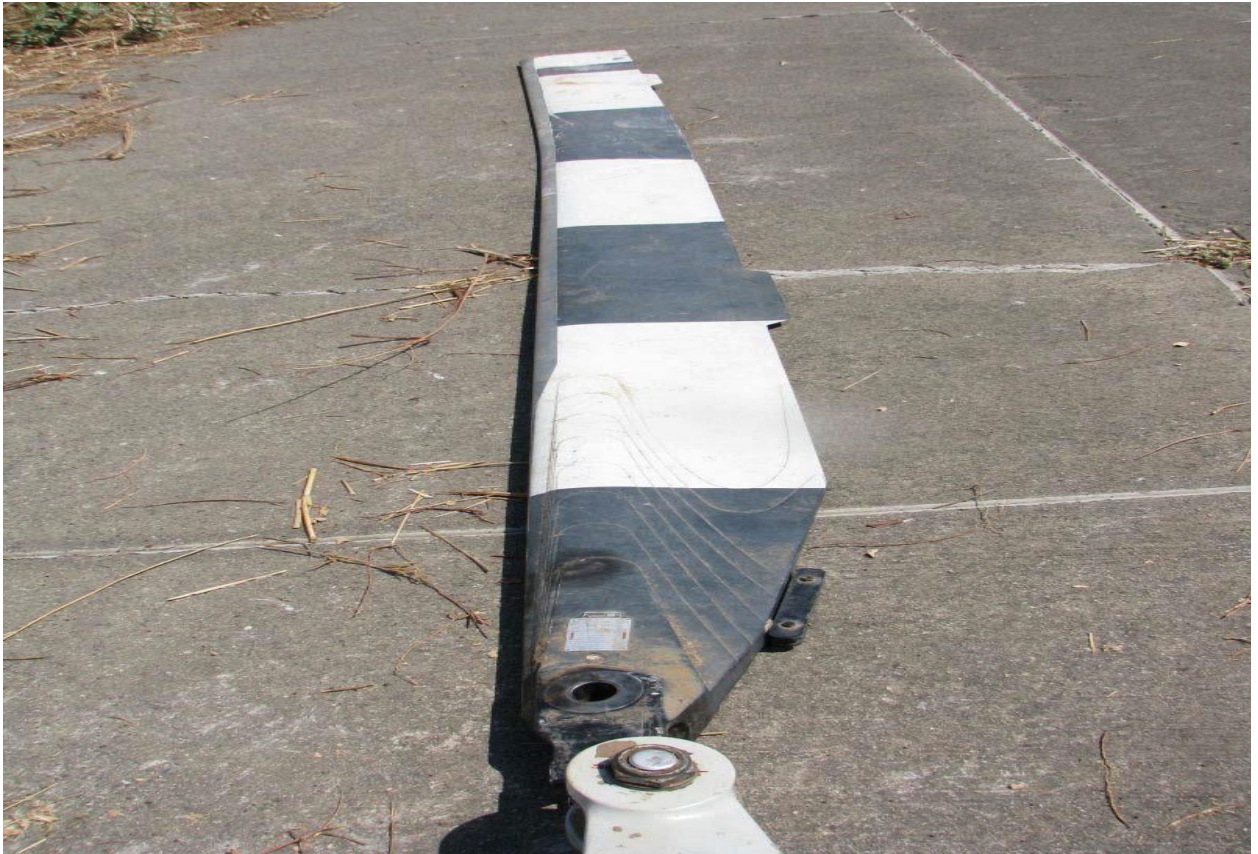
Picture19 Main rotor blade bent forward consistent with inertial forces when other blade struck round.
